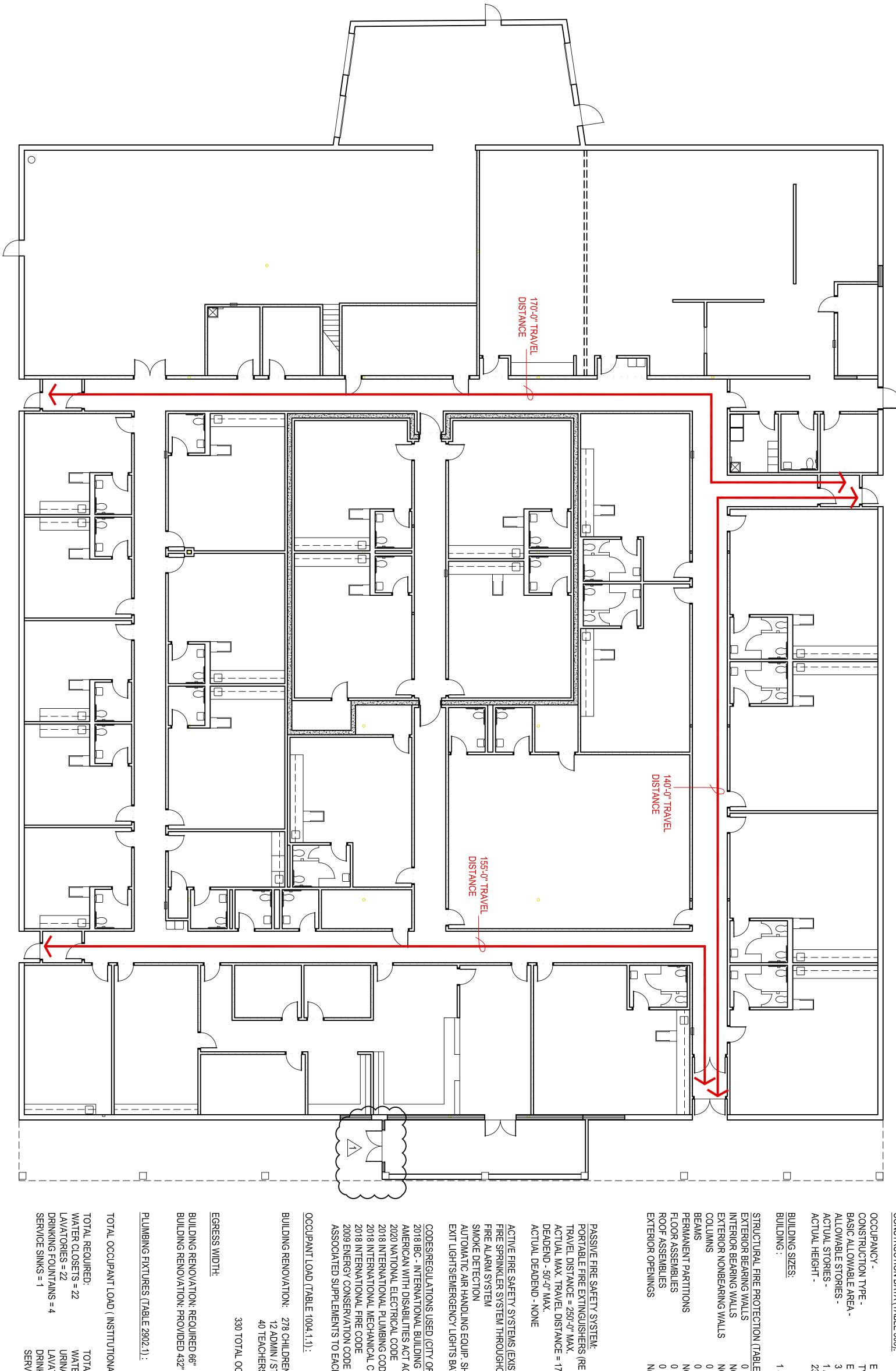
DENOTES 1 HR. RATED PARTITIONS CLOSE-OUT TO BOTTOM OF DECKING - CLOSE-OUT PARTITIONS TO BE CMU WHERE INDICATED ON STRUCTURAL FOR LOAD BEARING CONDITIONS. ALL OTHER INDICATED LOCATIONS TO BE CONSTRUCTED OF 1 LAYER OF 5/8" FIRE RATED GYP. BOARD EACH SIDE ON 6" METAL STUDS @ 16" O.C. STAGGER ALL JOINTS & PROVIDE FIRE TAPE. SEAL ALL PENETRATIONS W/ CONTINUOUS FIRE STOPPING INSULATION &/OR SEALANT.
