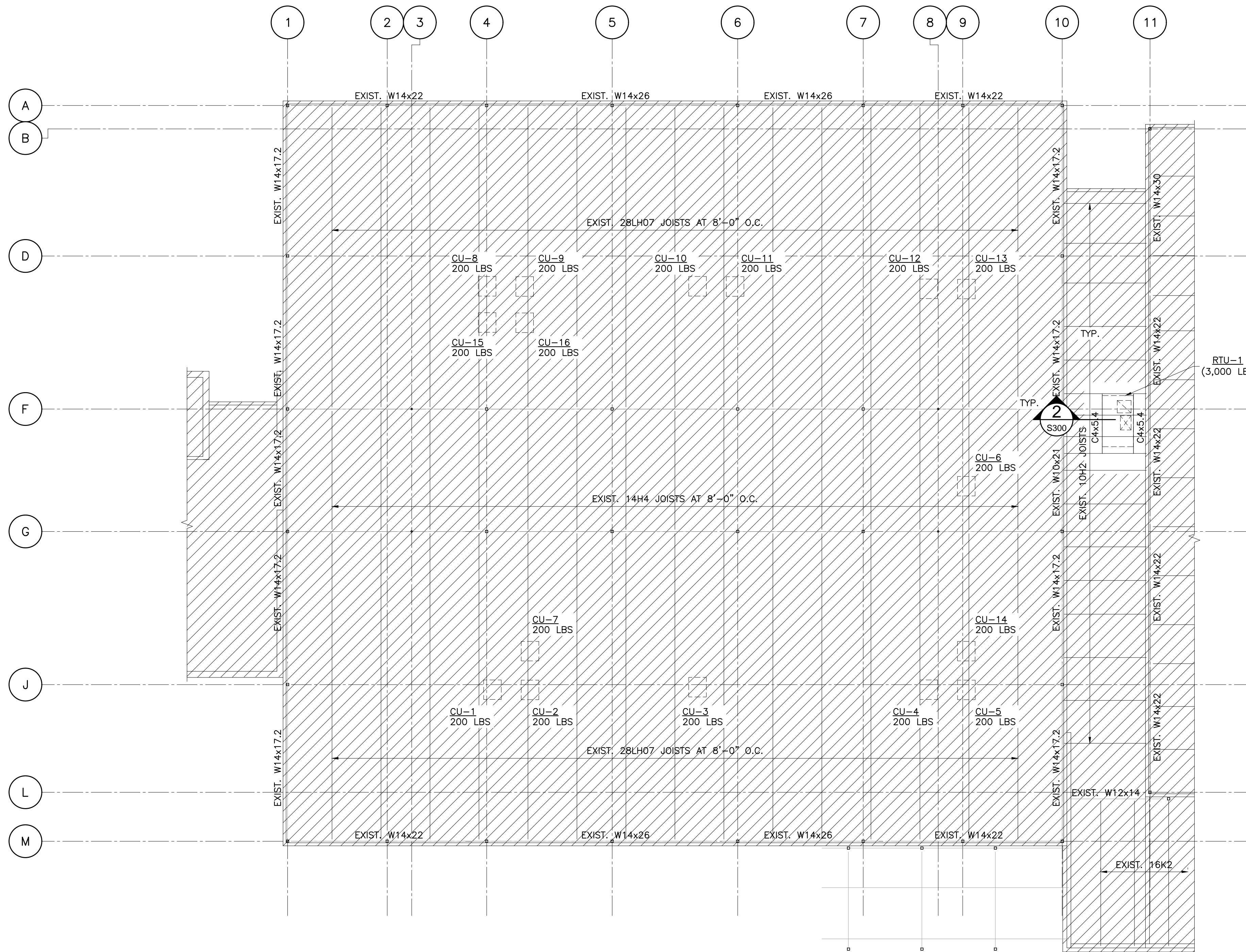
1 EXISTING ROOF FRAMING PLAN S300 SCALE: 3/32"=1'-0"
