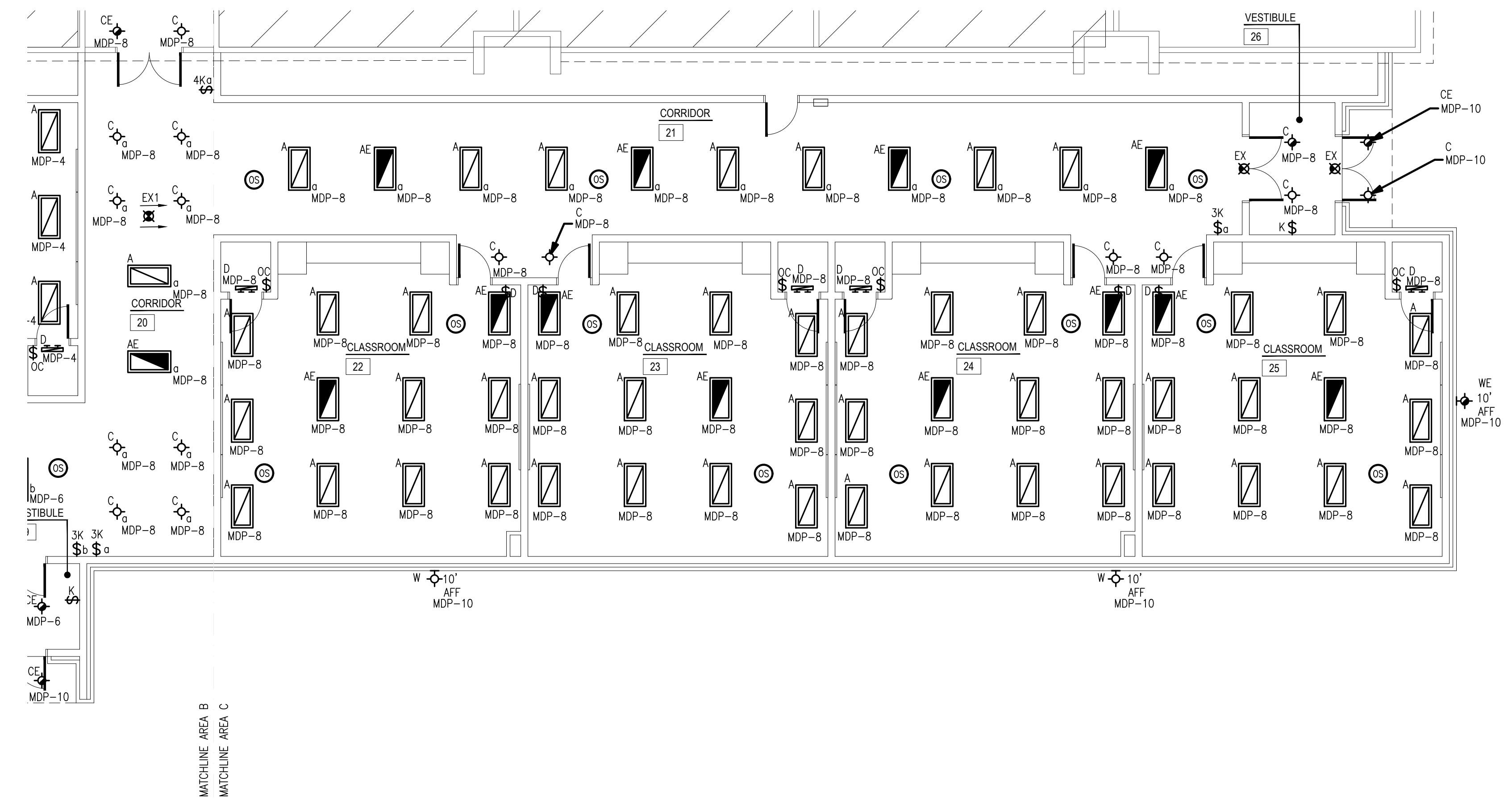
1 ELECTRICAL LIGHTING PLAN - AREA C SCALE: 1/8" = 1'-0"
